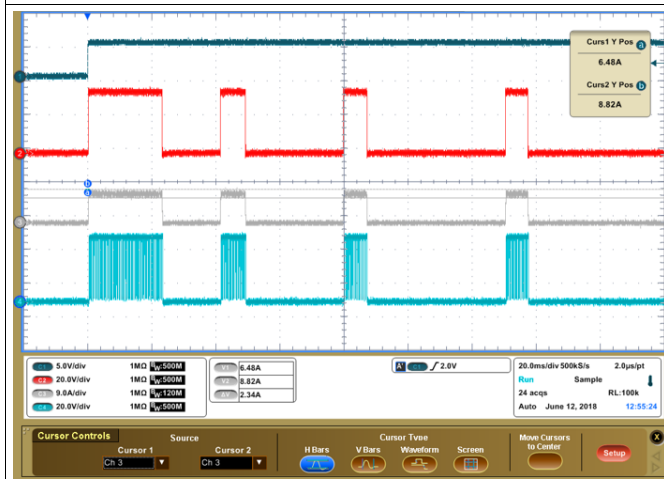
Figure 42. Overcurrent (OCP) Detection
