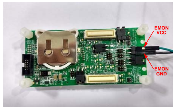
Figure 29. Board Setup for Downloading the Code
