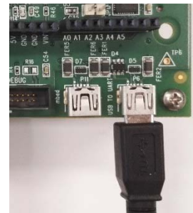
Figure 21. USB to UART Connection
