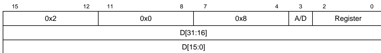
Figure 8-25. WAREG/WDREG Command Format
