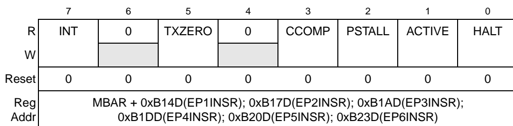
Figure 30-33. Endpoint n Status Register IN (EP n INSR)
