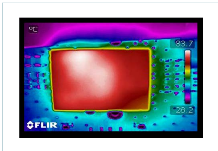
Figure 30 — Thermal image ( V_{IN} = 28V , I_{OUT} = 4.2A , CR, OLFM evaluation PCB)
