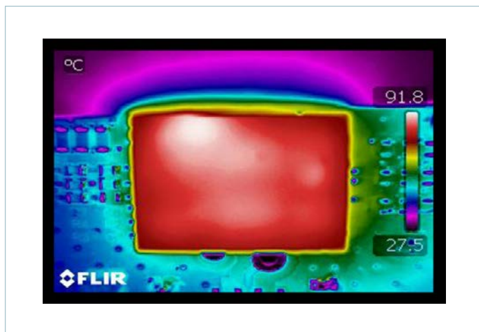
Figure 20 — Thermal image ( V_{IN} = 28V , I_{OUT} = 10A , CR, OLFM evaluation PCB)
