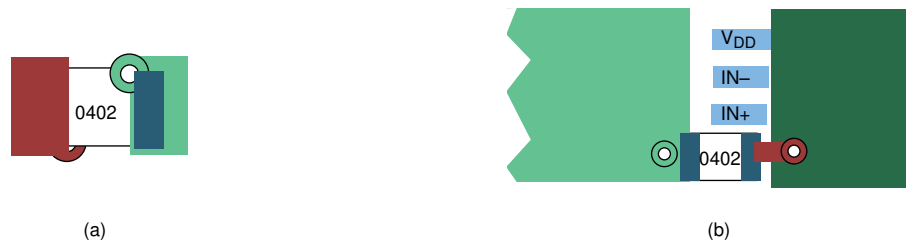
Figure 11-7. Typical Decoupling Capacitor Layouts
