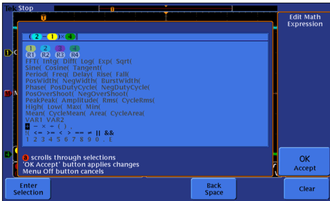
Figure 2. This menu lets you edit math expressions in the advanced math function of a DPO3034 digital oscilloscope.
