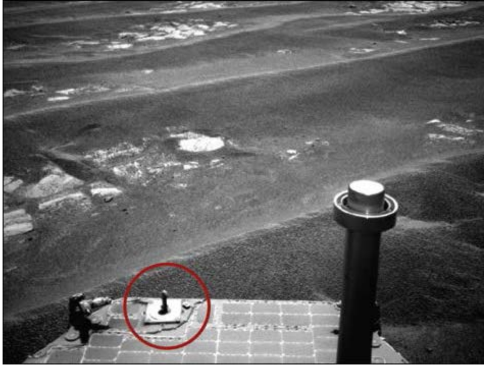
Figure 1. NASA's Mars Exploration Rover Opportunity used its navigation camera to record this view after completing a drive on July 17, 2011. The calibration standard (circled) was essential for the mission. Image courtesy of NASA/JPL-Caltec.
