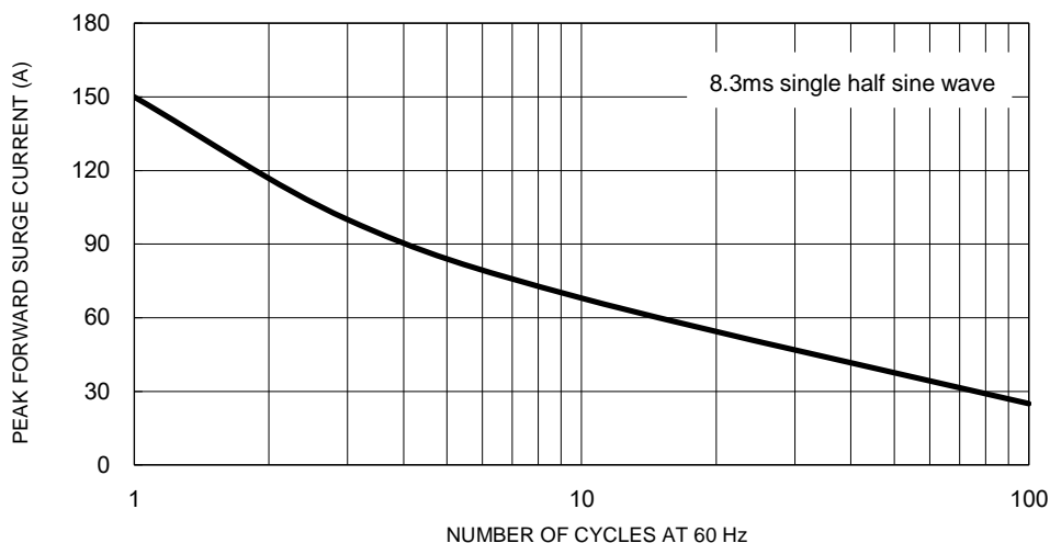
Fig.5 Maximum Non-Repetitive Forward Surge Current
